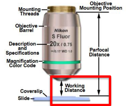
Figure 1 - Objective Working and Parfocal Distance
